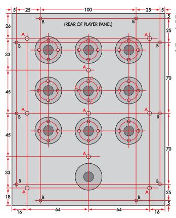
HOLES A: DRILLED 8mm INTO UNDERSIDE & TAPPED WITH A 4-40 UNC THREAD
