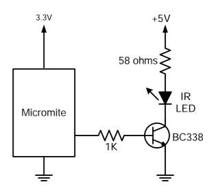
Note that the modulation frequency used is 38KHz and this matches the common IR receivers (described in the previous page) for maximum sensitivity when communicating between two Micromites.
