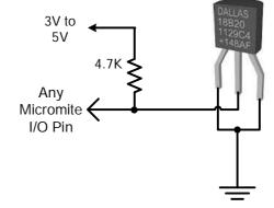
The time required for the overall measurement is 200mS and the running program will halt for this period while the measurement is being made. This also means that interrupts will be disabled for this period. If you do not want this you can separately trigger the conversion using the DS18B20 START command then later use the DS18B20() function to retrieve the temperature reading. The DS18B20() function will always wait if the sensor is still making the measurement.
