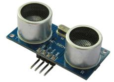
The I/O pins are automatically configured by this function but note that they should be 5V capable as the HC-SR04 is a 5V device. You can use multiple sensors connected to different I/O pins or even sharing the one trigger pin if care is taken to prevent one sensor from interfering with another.
