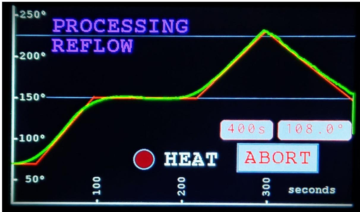
Please note: The initial flat section of the curve is set by 'Delay1' – to match the first ramp to the oven's capability. Whilst this might appear 'contrived' it isn't – as the remainder of the target curve is adjusted as necessary to suit the length of the preheat zone, etc.
