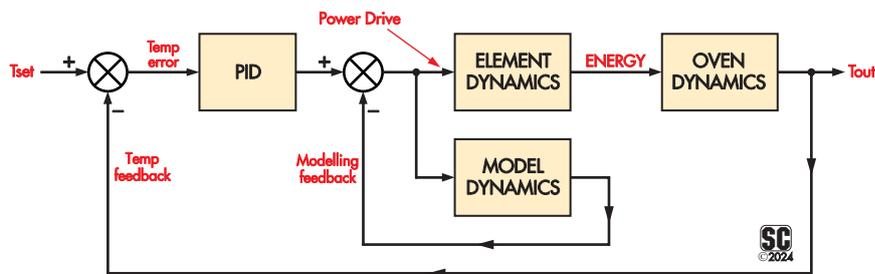
This system accumulates a 'count' of the energy provided to the elements, by adding an 'Energy Base' number, progressively decreased by a 'decay' factor to compensate for non-linearity, to the accumulator every ½ second while power is applied. This accumulated figure,  $E_{sum}$ , is then subtracted from the PID figure each cycle.
