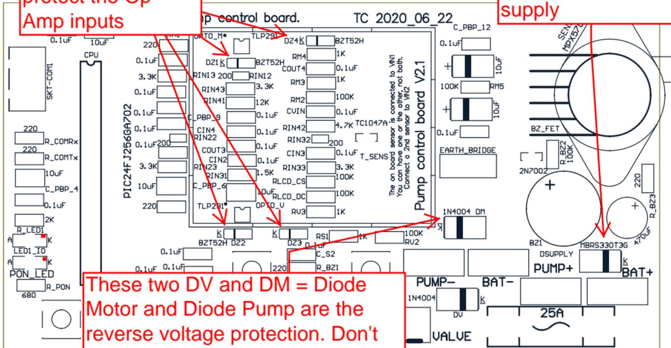
These two DV and DM = Diode Motor and Diode Pump are the reverse voltage protection. Don't need to be as big as DSUPPLY
