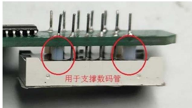
Once completed, and AFTER the two indicator LEDs, pushbutton and audio socket have been installed on the Main PCB, the display board may be mounted on the main PCB using the 10-way right-angle pin strip.
