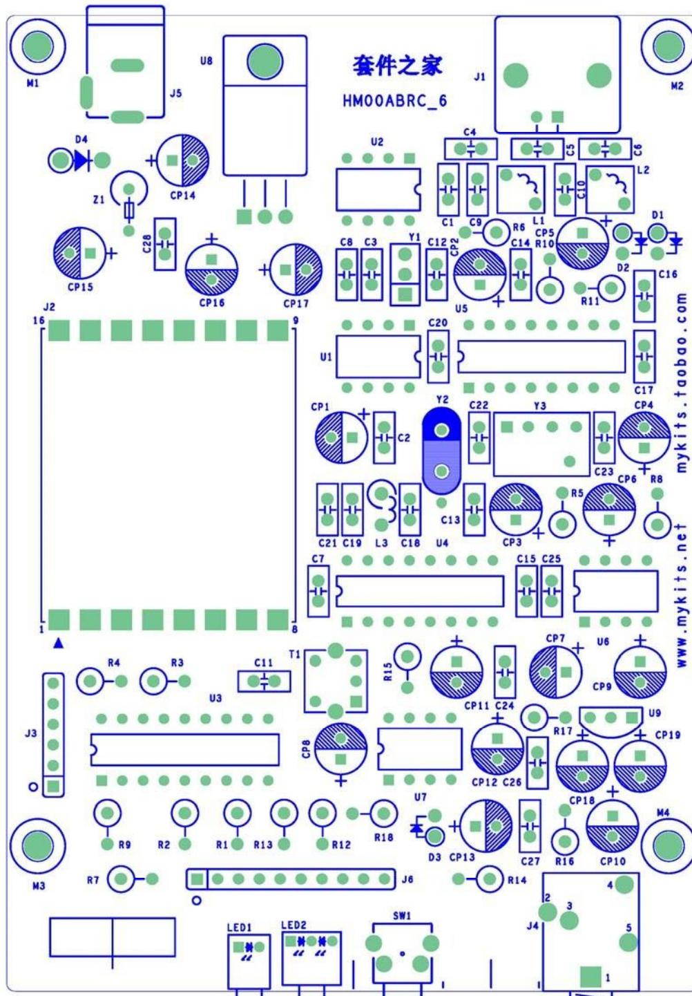
Please note pin 1 of Y1 (10.7MHz ceramic filter). It must be installed in the correct direction!
